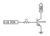
Switching circuit for the Propeller chip. Note HIGH signal required to turn on heater due to inversion of signal by the transistor.
