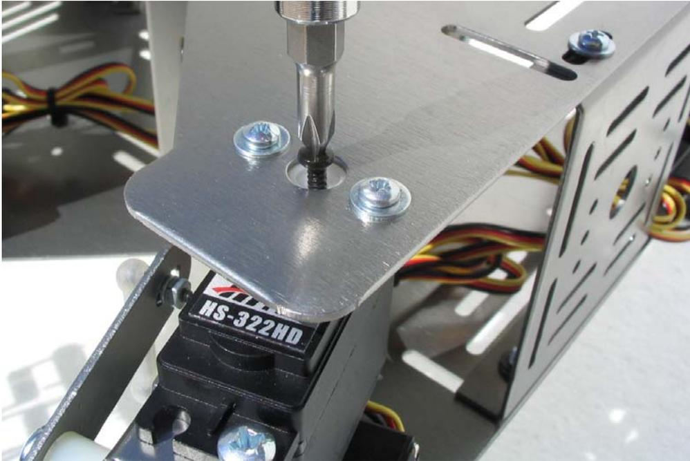
Figure 36: Securing the Leg Assembly
