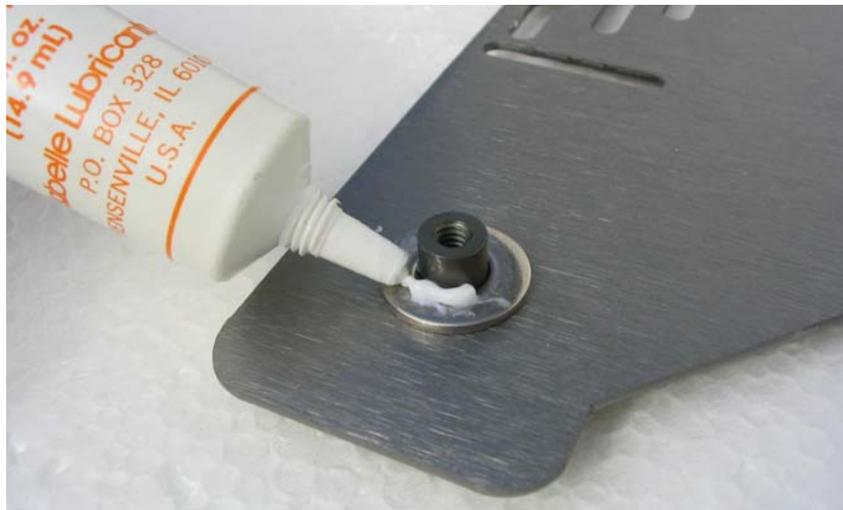
Figure 39: Grease Application – SAE Flat Washer
