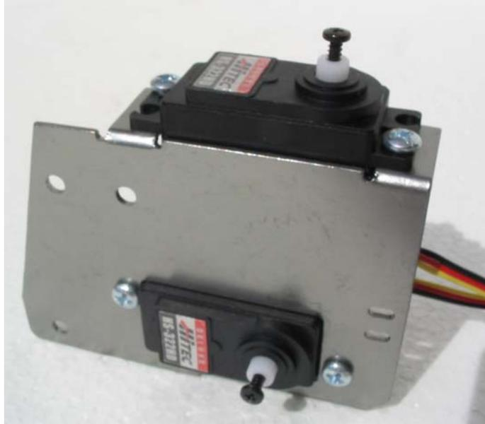
**Figure 5:** Completed Servo Installation – Front view
