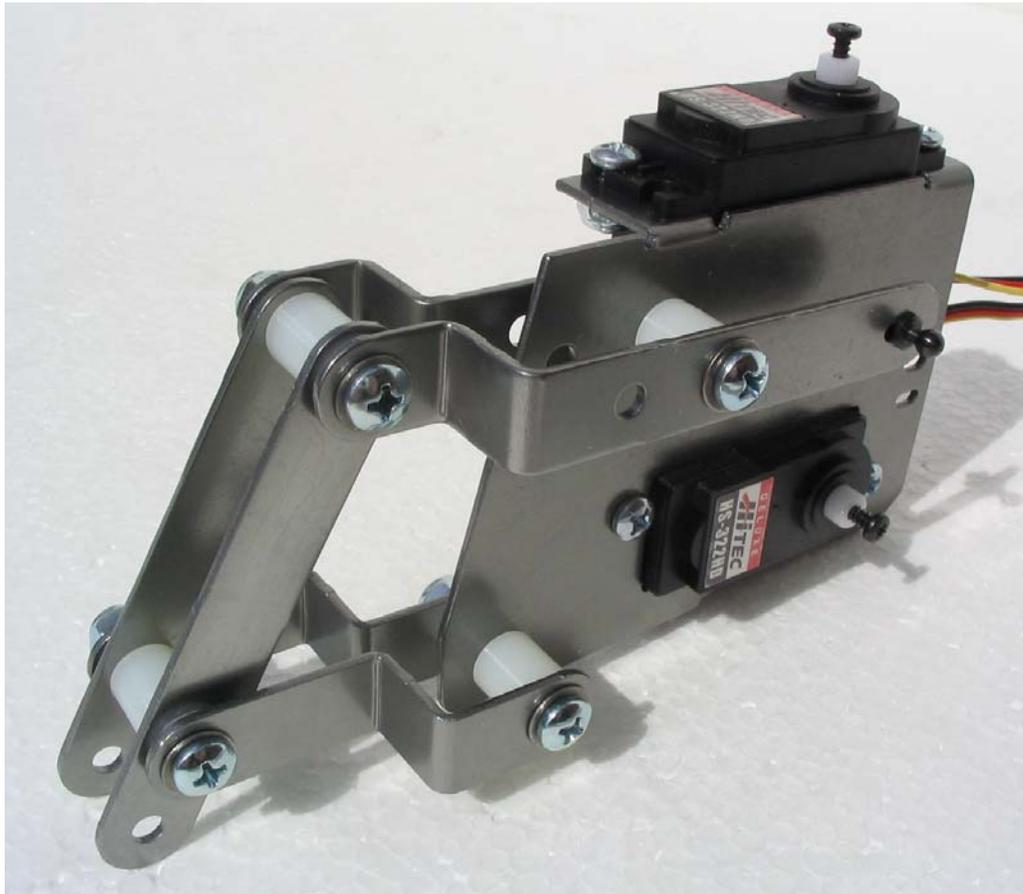
**Figure 20: Completed Leg Assembly**
