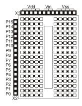
For chips with many legs (ICs), place them in the middle of the board so that half of the legs are on the left side and half are on the right side. Nodes on the left side are not connected to nodes on the right side.
